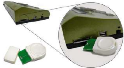
Figure 4: Illustration of the data stick and its insertion process into the eBraille panel
